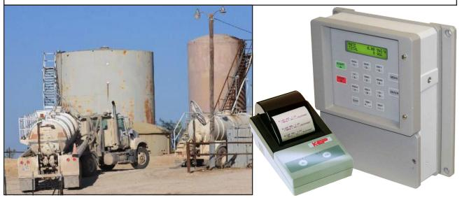
The produced water from either oil production or shale gas production wells is hauled away by a vacuum truck and disposed of at an authorized/approved disposal site. The trucks are lined up to dispose of the metered contents of their loads.
