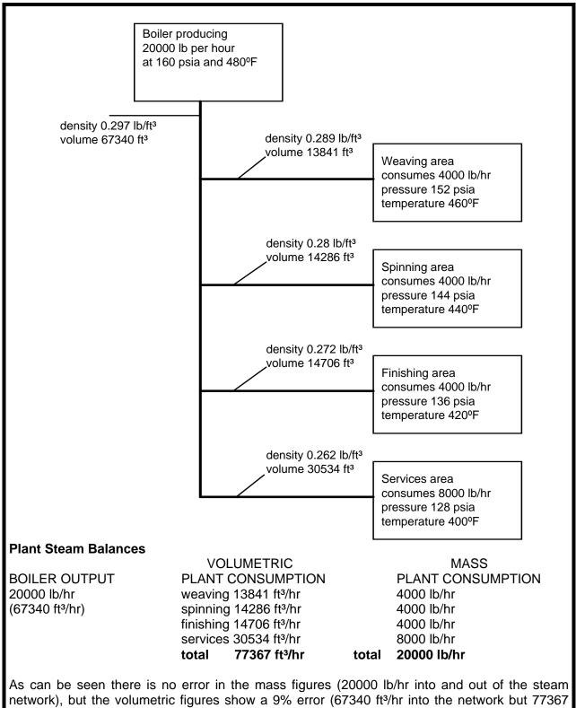
network), but the volumetric figures show a 9% error (67340 ft<sup>3</sup>/hr into the network but 77367 ft<sup>3</sup>/hr going out) The errors calculated here are conservative, actual figures on a plant are usually much worse.
