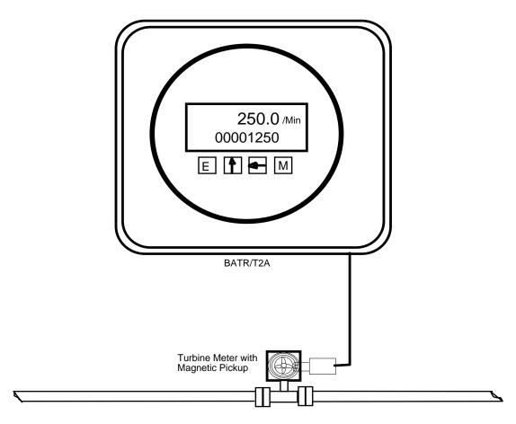
The BATR/T2A works well in this remote application because it is Battery powered and will monitor Rate of Flow and Total Flow without any external power source.
